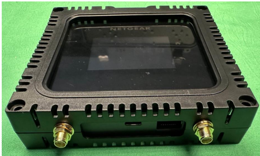
Figure 8: Secure the adapters using the washer and nut
