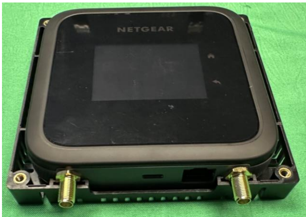
Figures 6-7: Installing the Router and Adapters to the M5-M6 Router Base and Cover
