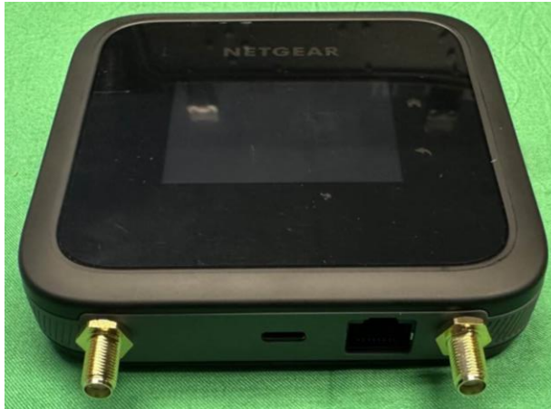
Figure 5: Installing the SMA(F) – TS9(M) Adapters
