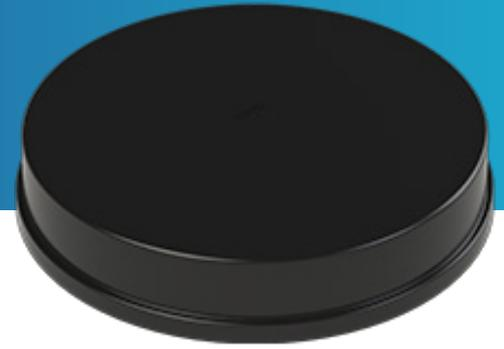
The Husky PRO Series antenna is designed for high performance. The Husky provides up to 8 WIFI connections and GPS. This rugged omni-directional antenna works on all the common North American LTE bands with high efficiency. Also supports CBRS and LAA. The antenna requires a single 1.5-inch mounting hole. Optional magnetic mount allows mounting on a steel surface without mounting holes.
