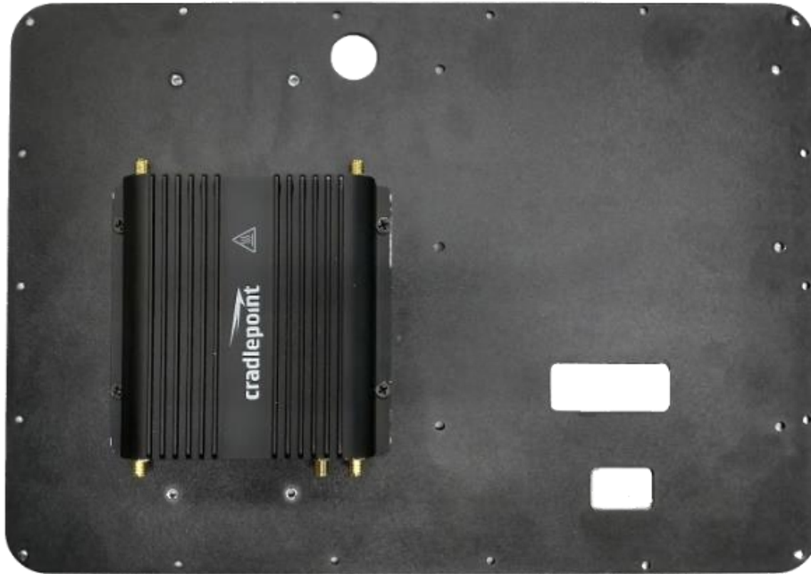
Figure 3: Fasten the router to the cover plate using PTA0368-B screws. (Beagle L)
