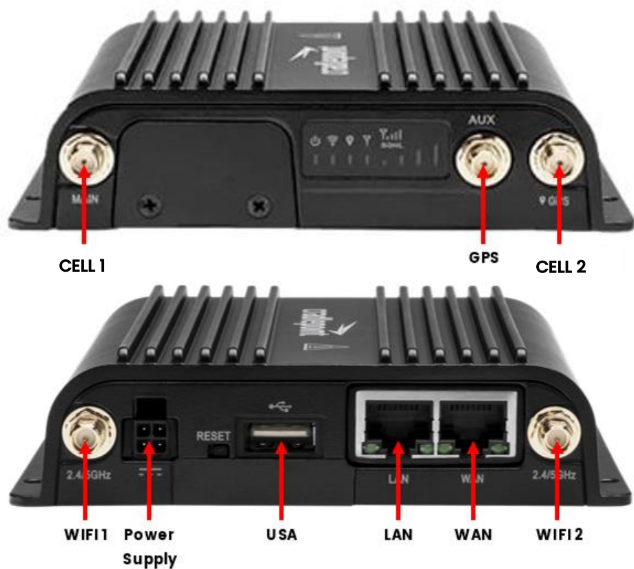
Figure 7: Cradlepoint IBR600, IBR900, & R500-PLTE Connections
