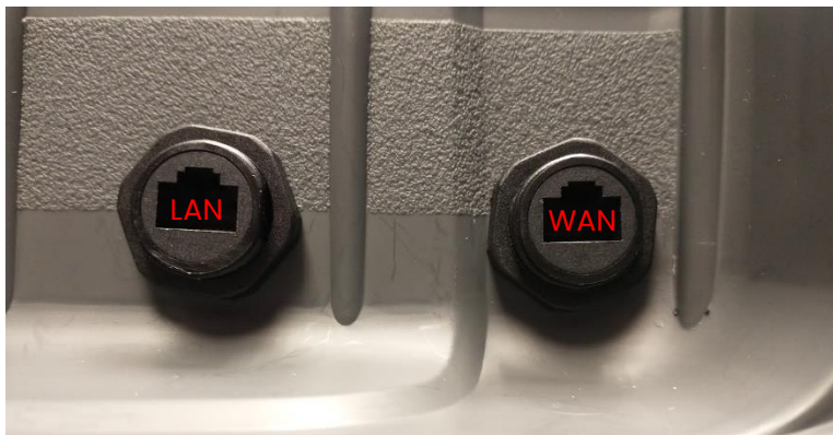
Figure 8: Connect the router to the RJ-45 ports on the case using ethernet cords.
