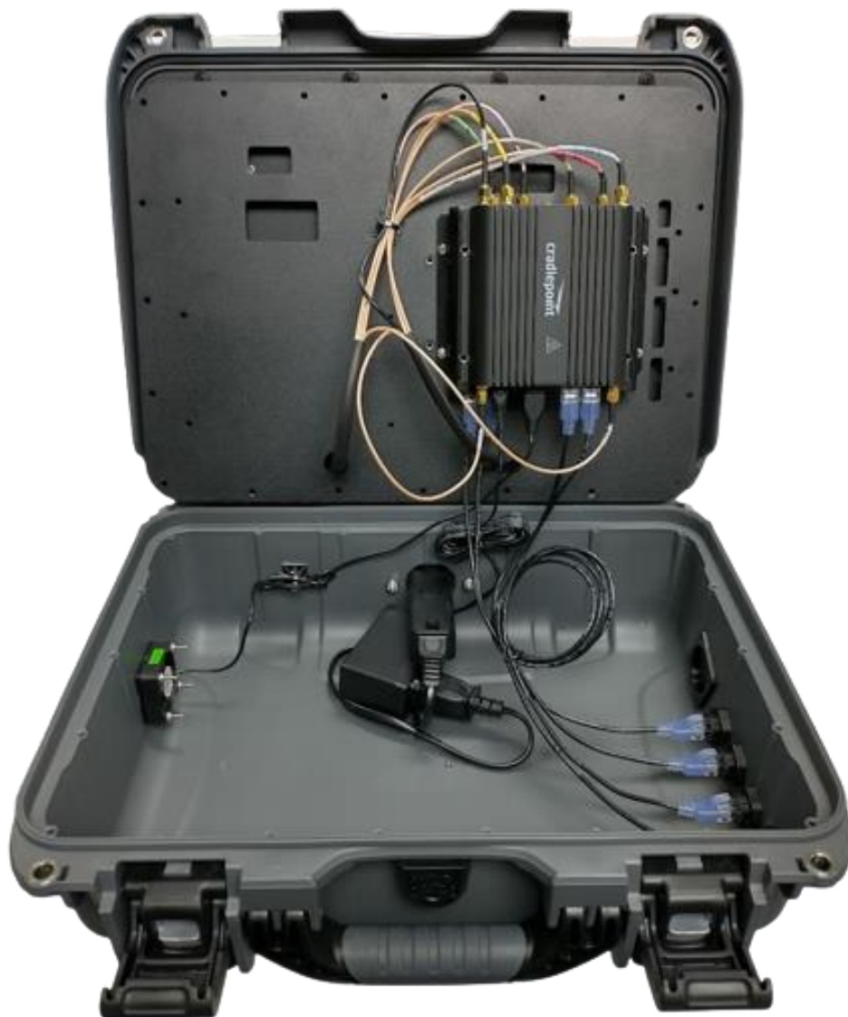
Figure 13: Fully Connected 9in1 Bernese Mountain Dog L with Cradlepoint IBR900 Router and COR Extensibility Dock
