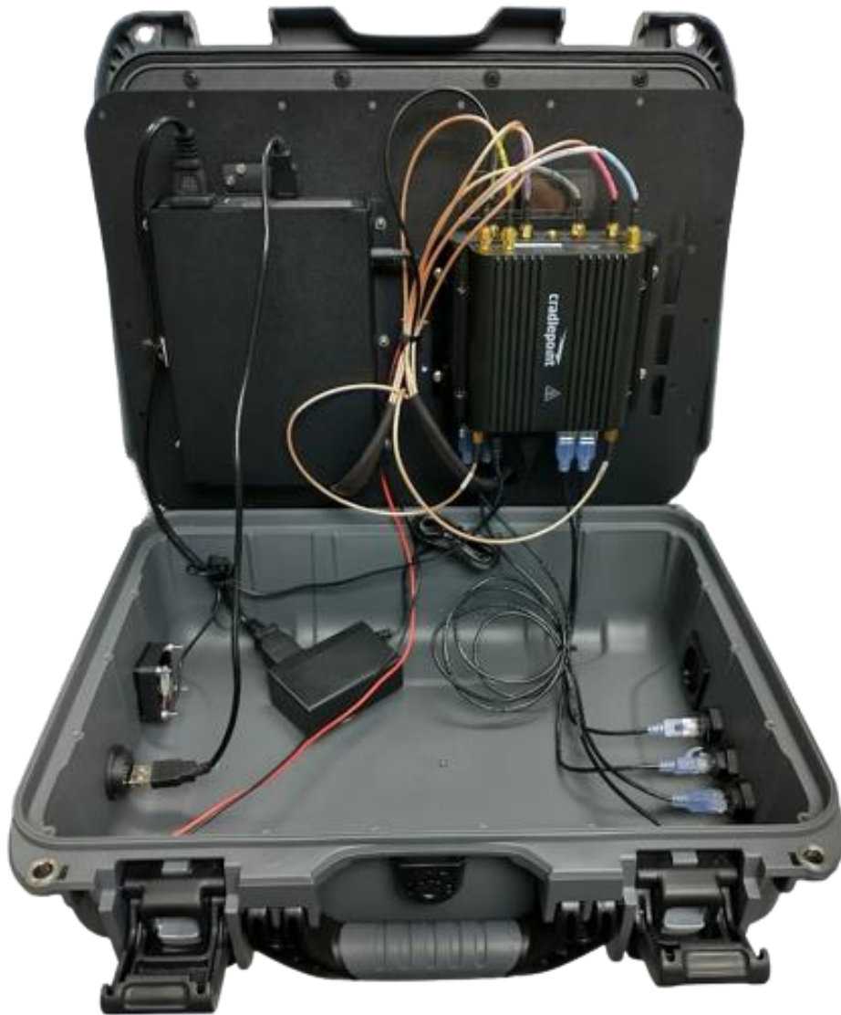
Figure 12: Fully Connected 9in1 Bernese Mountain Dog G with Cradlepoint IBR900 Router and COR Extensibility Dock
