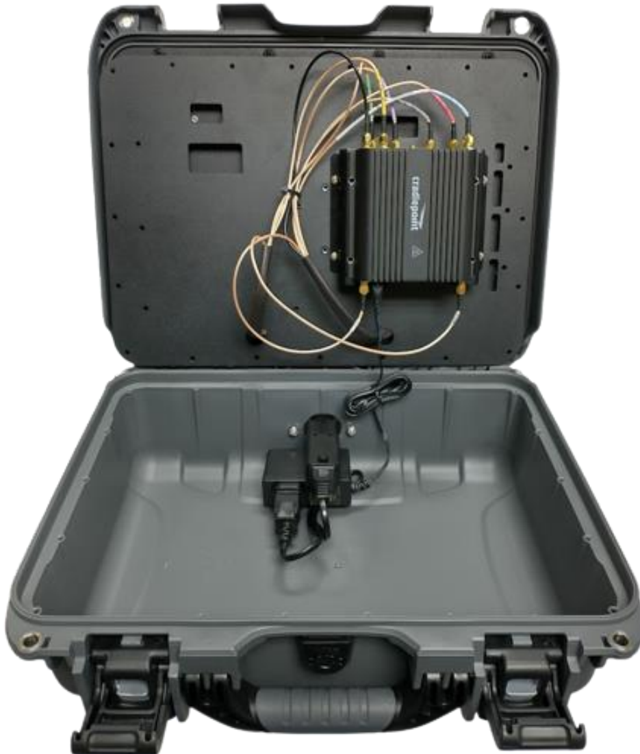
Figure 11: Fully Connected 9in1 Bernese Mountain Dog A with Cradlepoint IBR900 Router and COR Extensibility Dock
