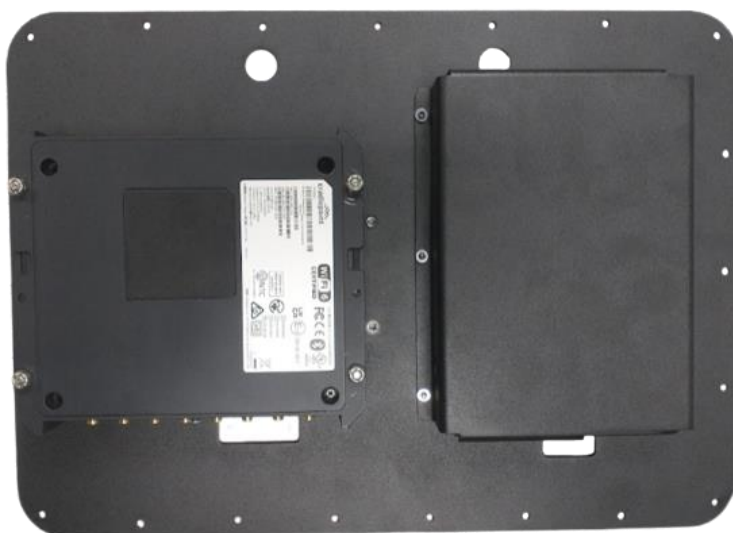
Figure 4: For R1900 router, fasten the router to the cover plate PTA0579 screws, PTA0140 washers, PTA0844 lock washers, and PTA0408 nuts.
