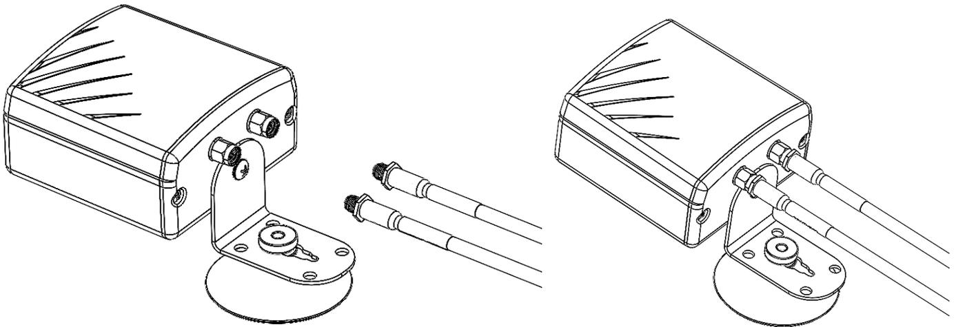
4. Using the suction cup, mount the antenna on a glass window on the interior face at least 24 inches away from other devices or obstructions.
