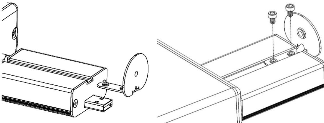
4. Fasten the wall mount bracket to the router bracket using the provided 8-32 machine screw.
