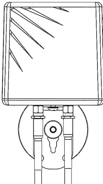
5. Secure the antenna cables roughly 6 inches below the antenna to provide strain relief. Vinyl electrical tape or cable-ties can be used. If using cable-ties outside, make sure to use UV resistant cable-ties.
