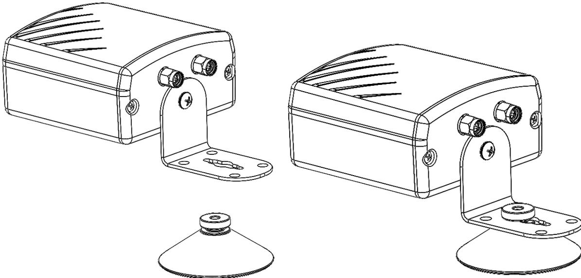
3. Connect the SMA(F) ends of the cables in the SMA(M) to SMA(F) cable kit to the connectors on the antenna.
