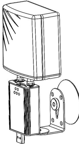
6. Using the suction cup, mount the antenna on a glass window on the interior face at least 24 inches away from other devices or obstructions.
