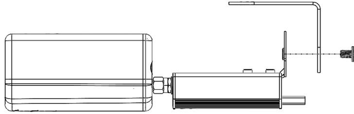
5. Insert the provided suction cup into the keyhole slot on the wall mount bracket.
