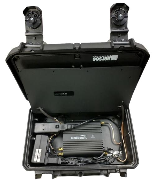
Figure 9: Fully Connected 5in1 Golden Retriever A with Cradlepoint IBR900 Router
