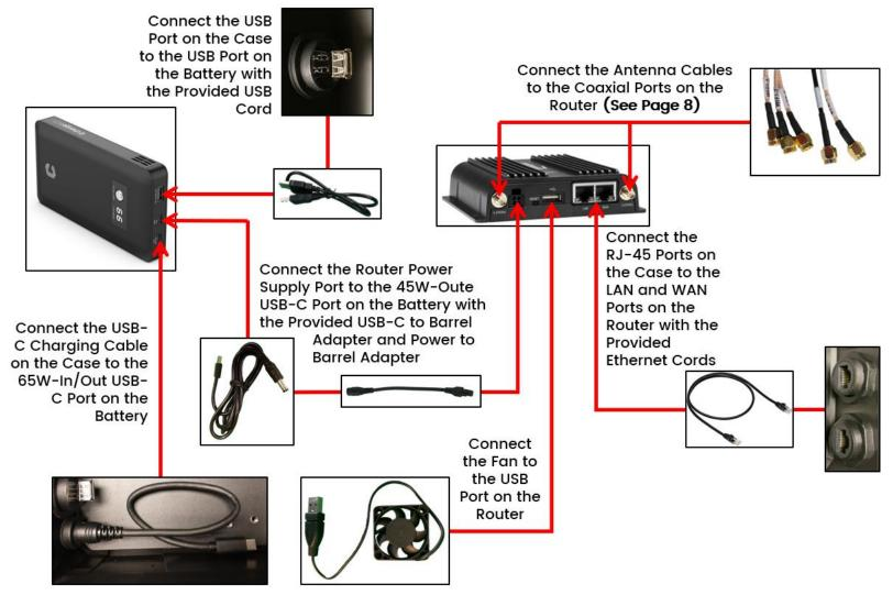
Figure 5: Connection Diagram for Golden Retriever G
