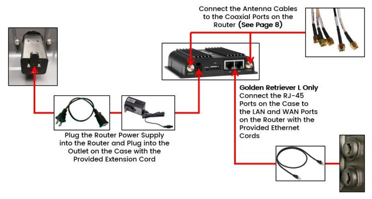
Figure 4: Connection Diagram for Golden Retriever A & L
