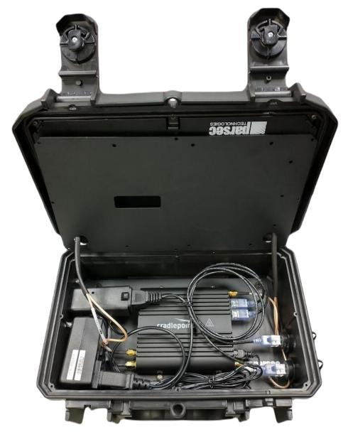
Figure 11: Fully Connected 5in1 Golden Retriever L with Cradlepoint IBR900 Router
