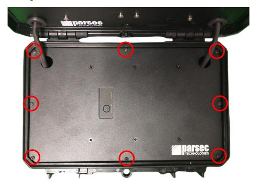
Figure 12: Fasten the cover plate to the case using PTA0071B screws.
