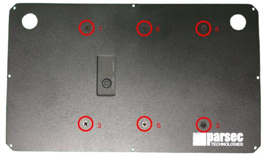
Figure 2: Fasten the battery tray with battery pack to the cover plate using PTA0368-B screws. (Golden Retriever G)
