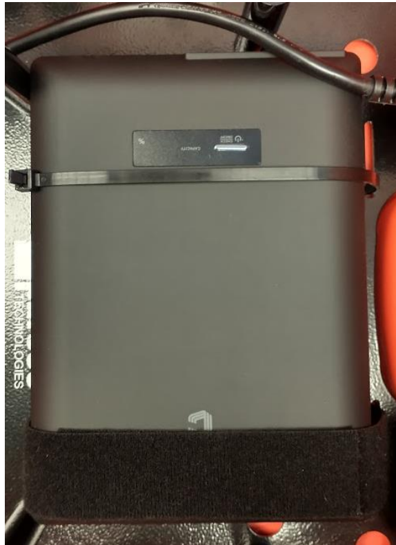
Figure 2: Strap the battery pack down to the base plate.
