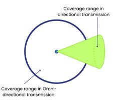
When selecting the location of a directional antenna, ensure that the antenna can be mounted in such a way that it faces the desired signal source, typically the nearest cell tower.
