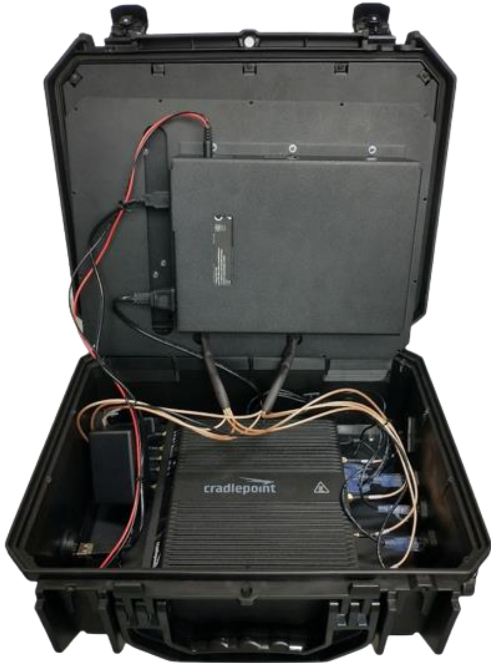
Figure 11: Fully Connected 9in1 St. Bernard G with Cradlepoint IBR1700 Router
