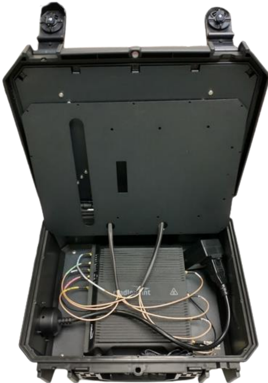
Figure 10: Fully Connected 9in1 St. Bernard A with Cradlepoint IBR1700 Router
