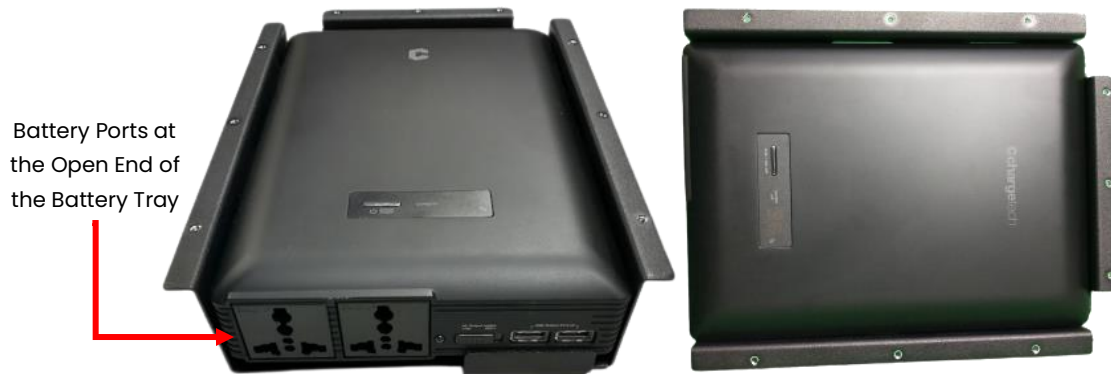
Figure 2: Place the ChargeTech battery pack into the battery tray. (St. Bernard G)
