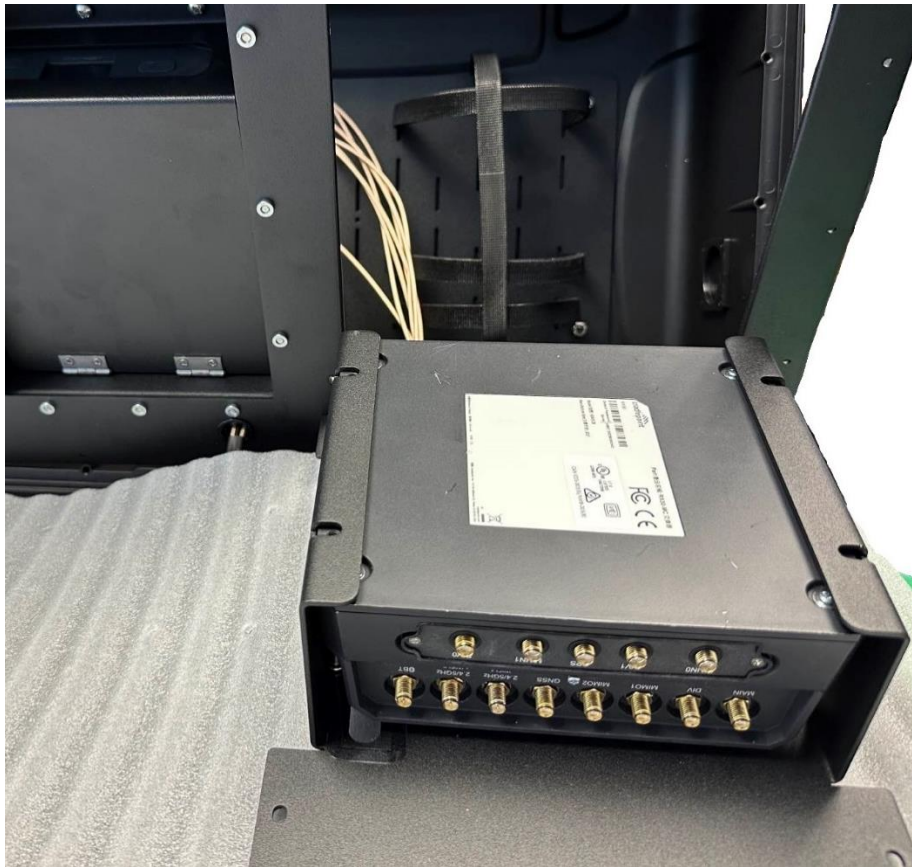
Figure 6: Insert the R1900 Router into the Router Module.
