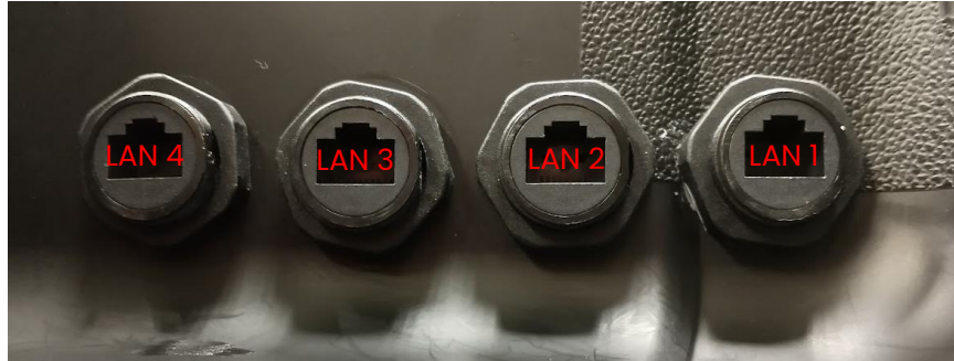
Figure 12: Connect the router to the RJ-45 ports on the case using ethernet cords.
