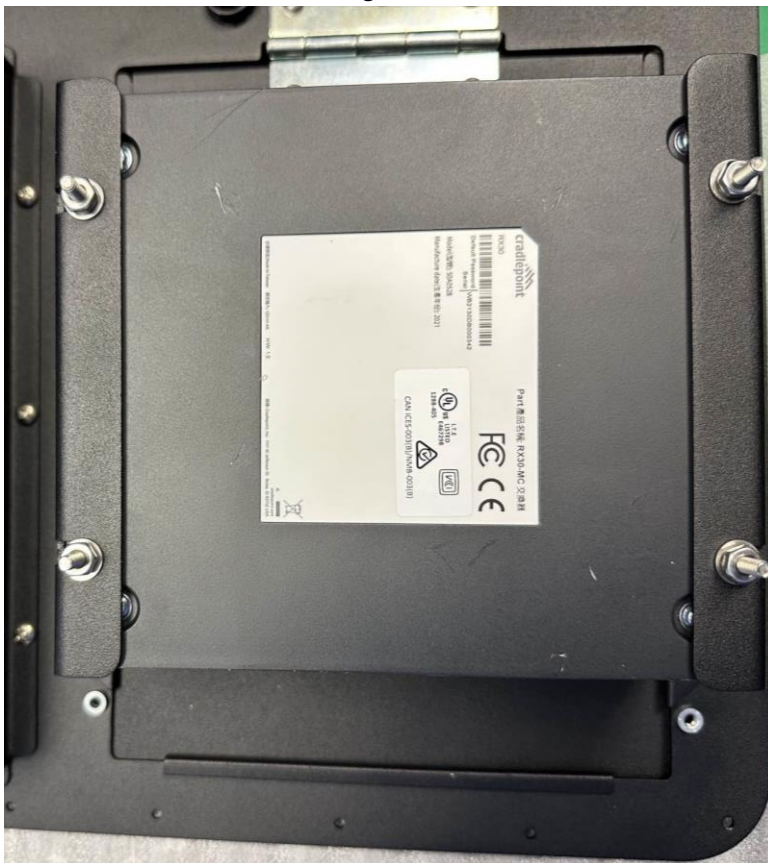
Figure 7: Mount the R1900 Router to the Cover Plate.
