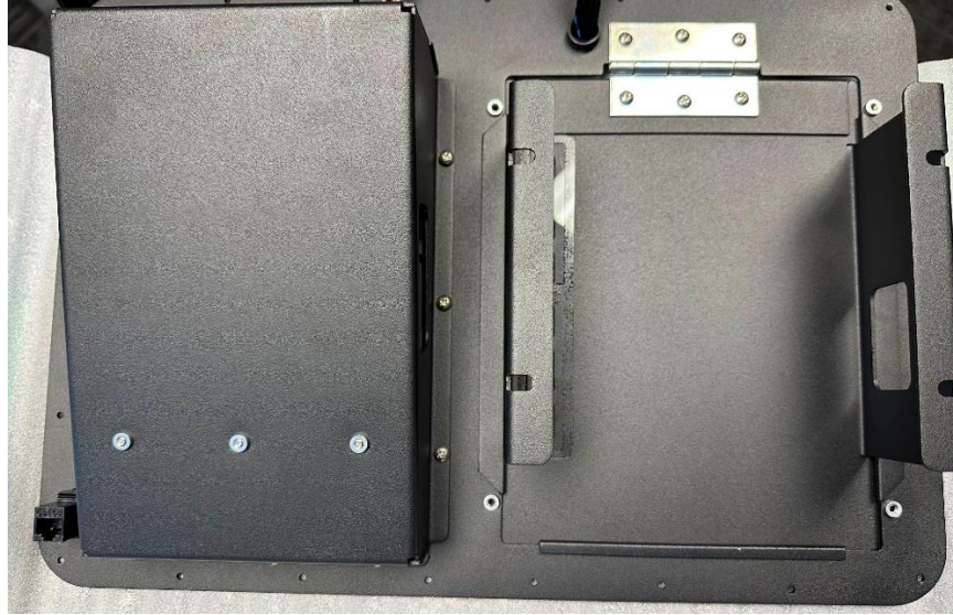
Figure 4: Place the Cover Plate on the Antenna Plate.
