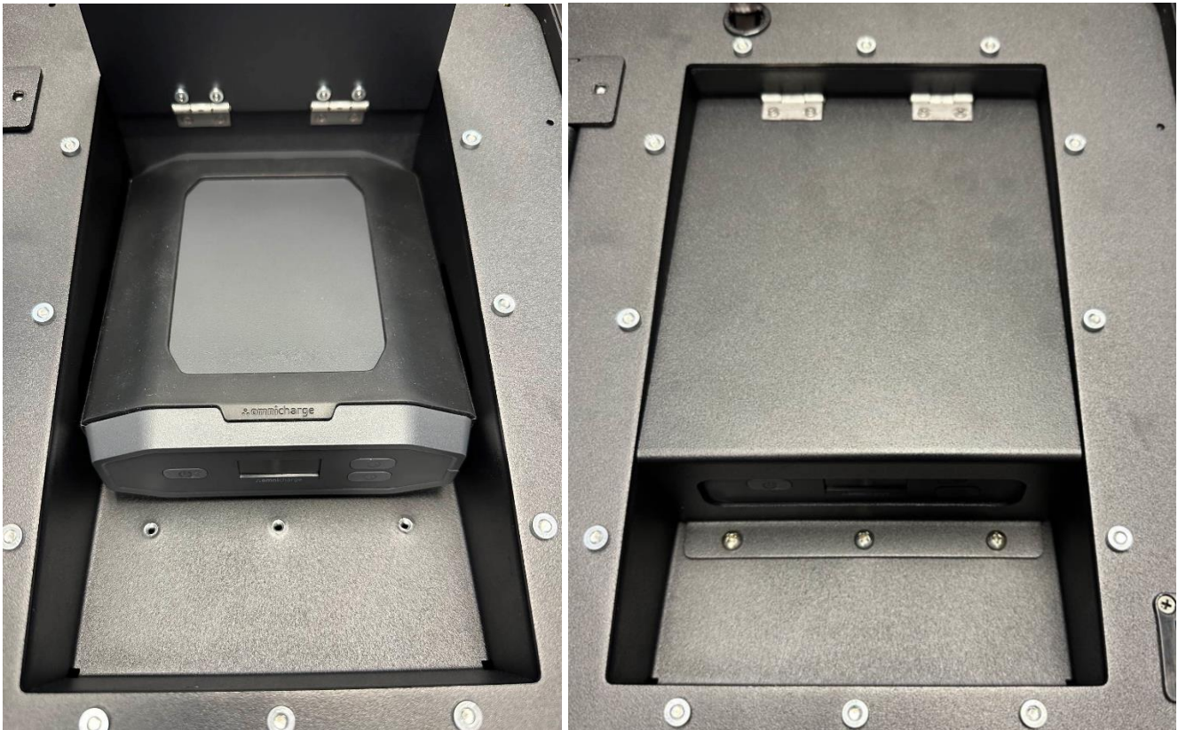
Figures 2-3: Insert the battery pack into the battery tray and secure the Battery Tray.
