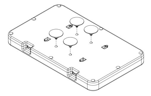
3. Install the Antenna on the Window. Ensure the antenna is upright, as shown below.
