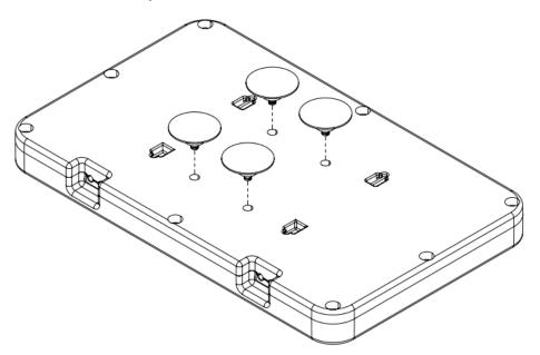
3. Install the Antenna on the Window. Ensure the antenna is upright, as shown below.
