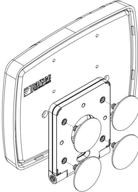
3. Use the PTA0916 5mm Allen Key to loosen the Desk Mount Bracket and enable it to rotate. Ensure the antenna is upright, as shown below.
