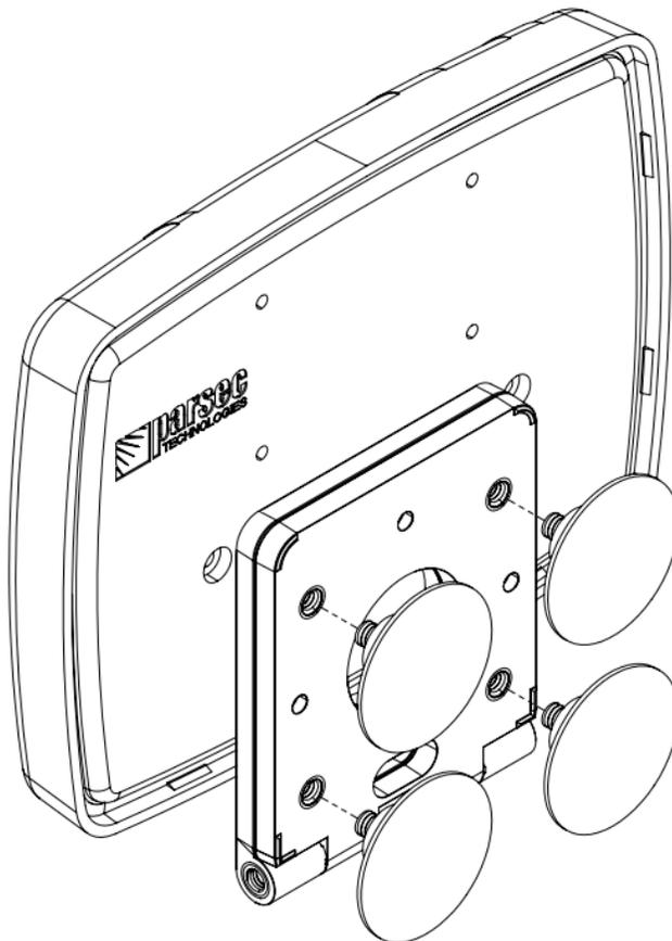
3. Install the Antenna on the Window. Ensure the antenna is upright, as shown below.
