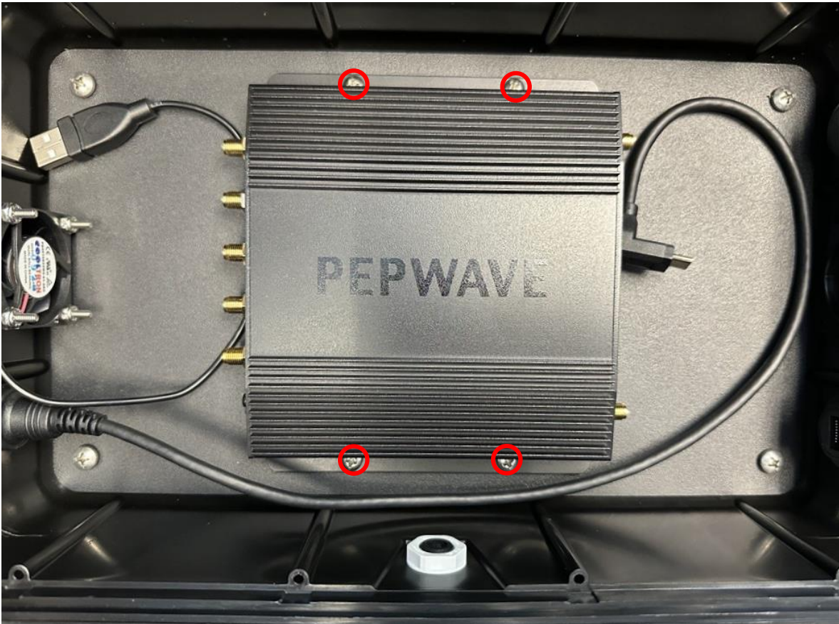
Figure 3: Fasten the router to the bottom plate using PTA0399-TL screws.
