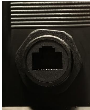
Figure 8: Connect the router to the RJ-45 ports on the case using ethernet cords.
