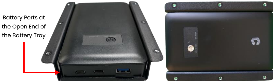
Figure 1: Place the ChargeTech battery pack into the battery tray. (Boxer G)
