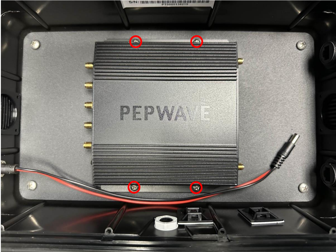
Figure 4: Fasten the router to the bottom plate using PTA0399-TL screws.
