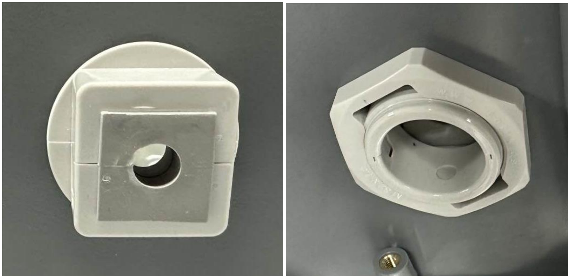
Figures 13-14: Removing the Cable Gland from the Dalmatian
