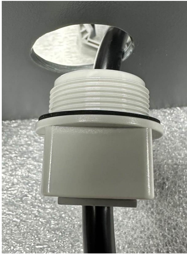
Figure 23: Installing the gasket on the cable gland
