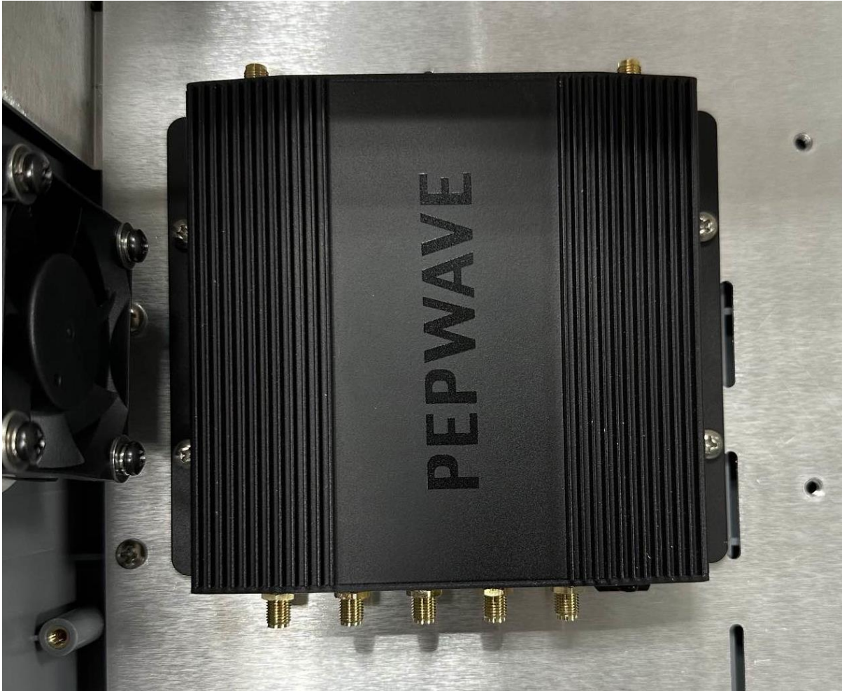
Figure 11: Peplink MAX BR1 Pro Router Installation
