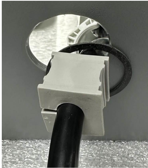
Figure 20: Installing the cable grommet on the cable
