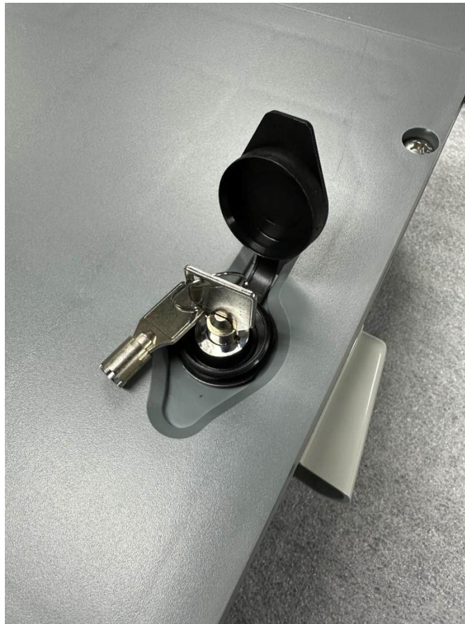
Figure 36: Lock the lid to the enclosure
