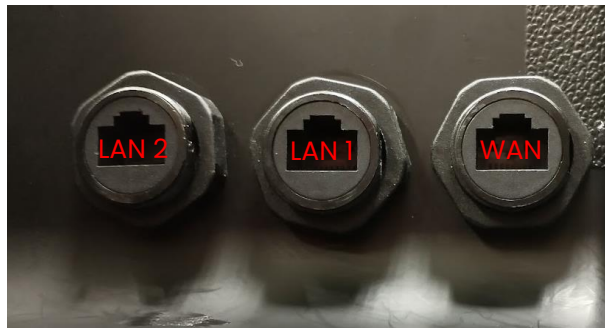
Figure 23: Connect the router to the RJ-45 ports on the case using ethernet cords.
