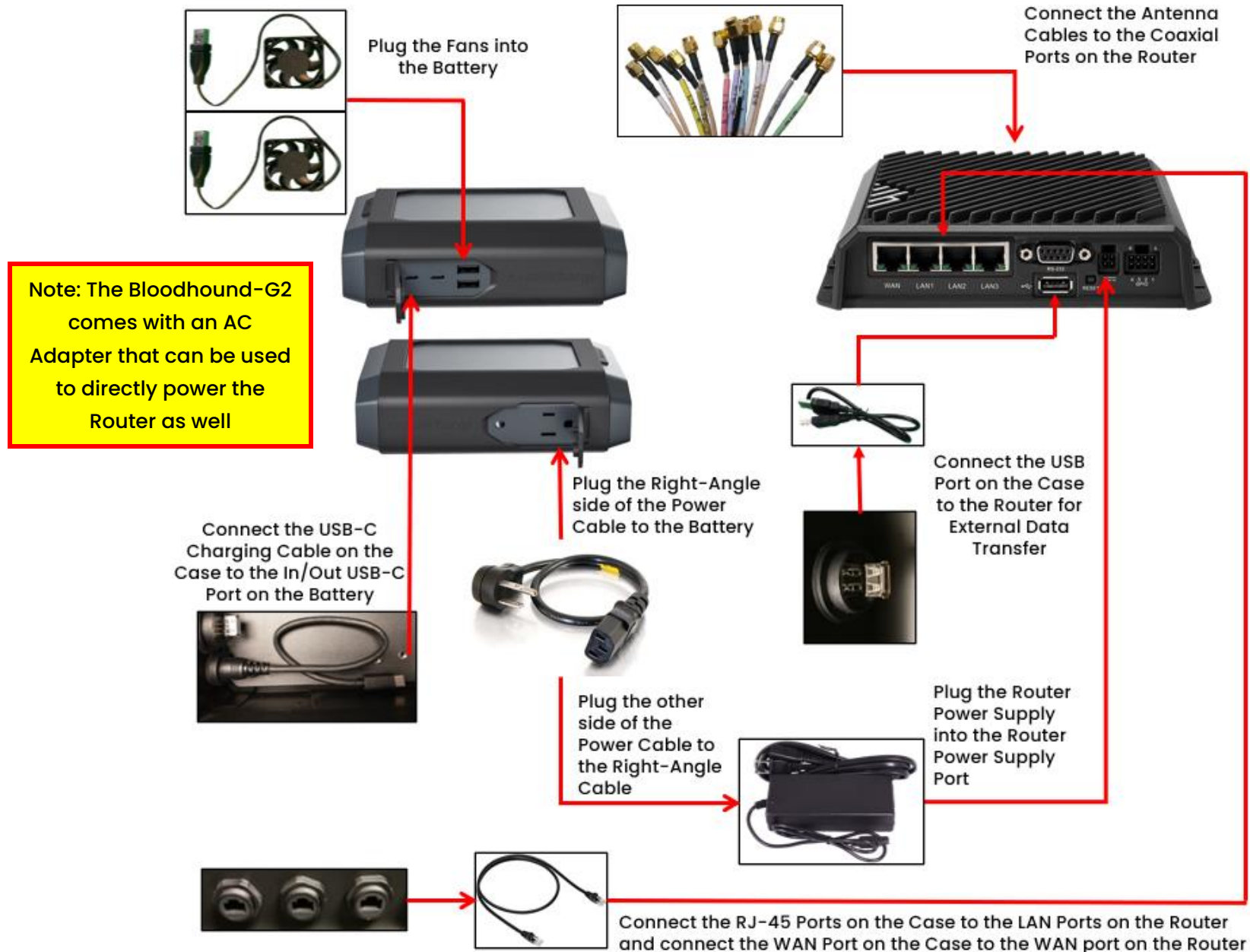
Figure 10: Connection Diagram for Bloodhound G2
