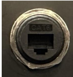
Figure 6: Connect the router to the RJ-45 ports on the case using ethernet cords.
