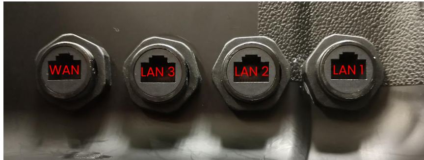
Figure 10: Connect the router to the RJ-45 ports on the case using ethernet cords.
