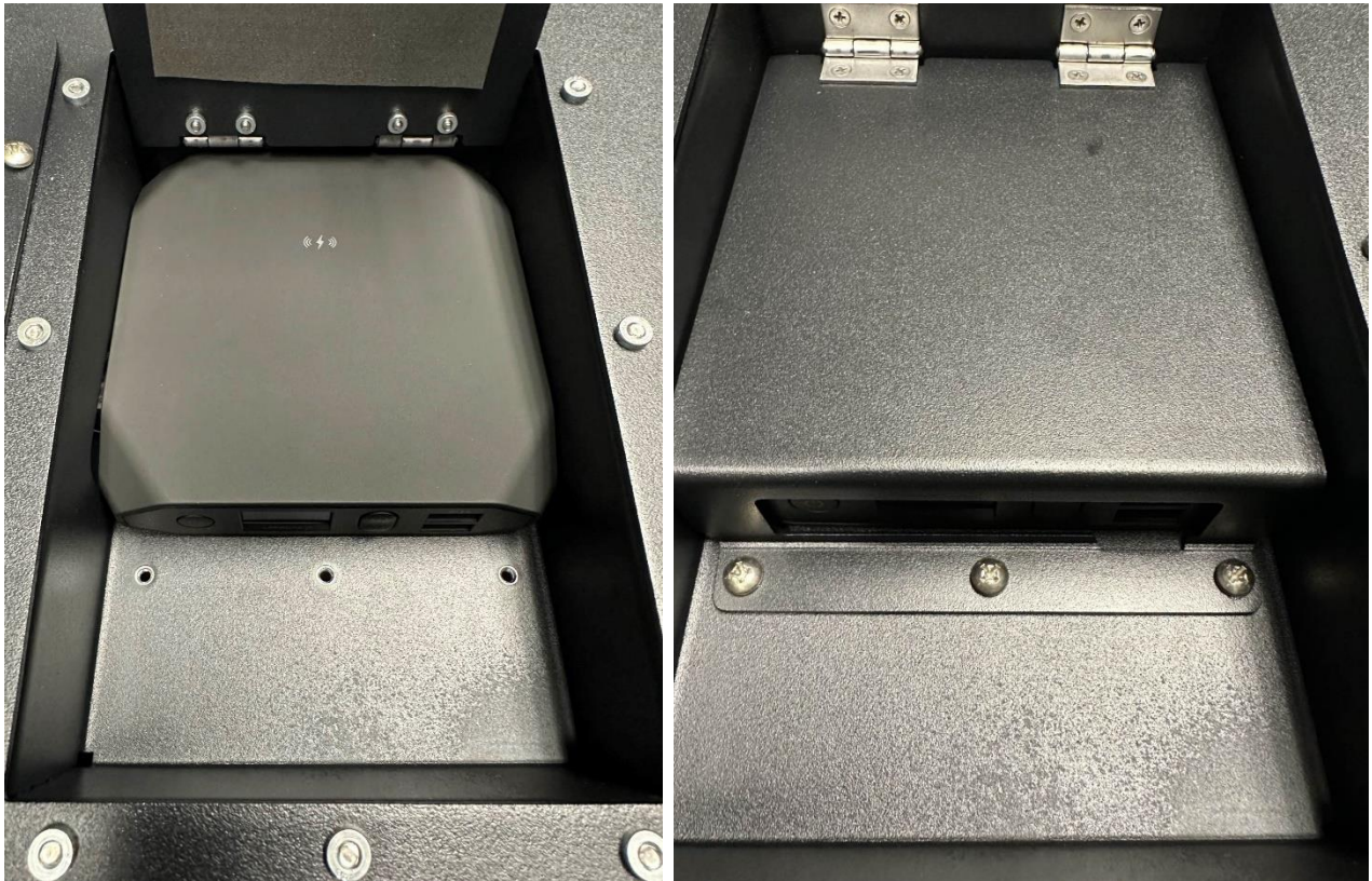
Figures 1-2: Insert the battery pack into the battery tray and secure the Battery Tray.
