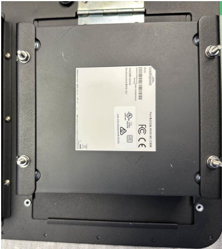
Figure 9: Mount the R1900 Router to the Cover Plate.
