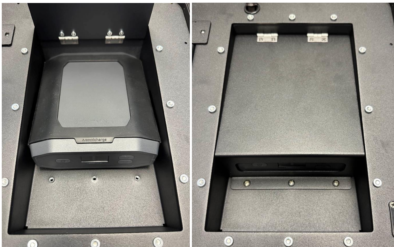
Figures 2-3: Insert the battery pack into the battery tray and secure the Battery Tray.
