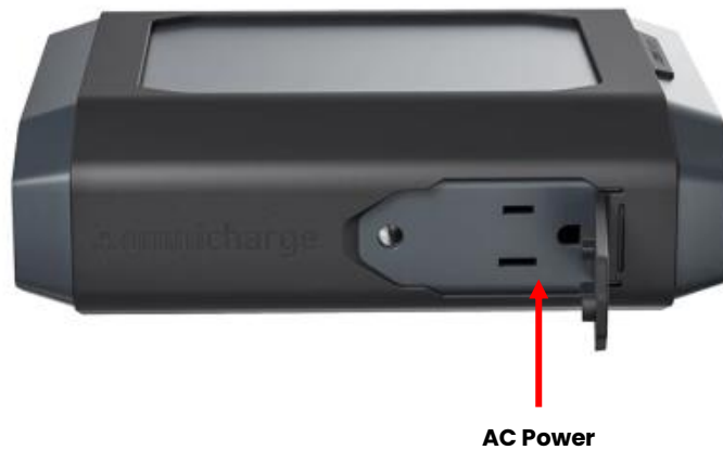
Figure 12: Omnicharge Ultimate 38k Battery Pack Connections (Left Side).
