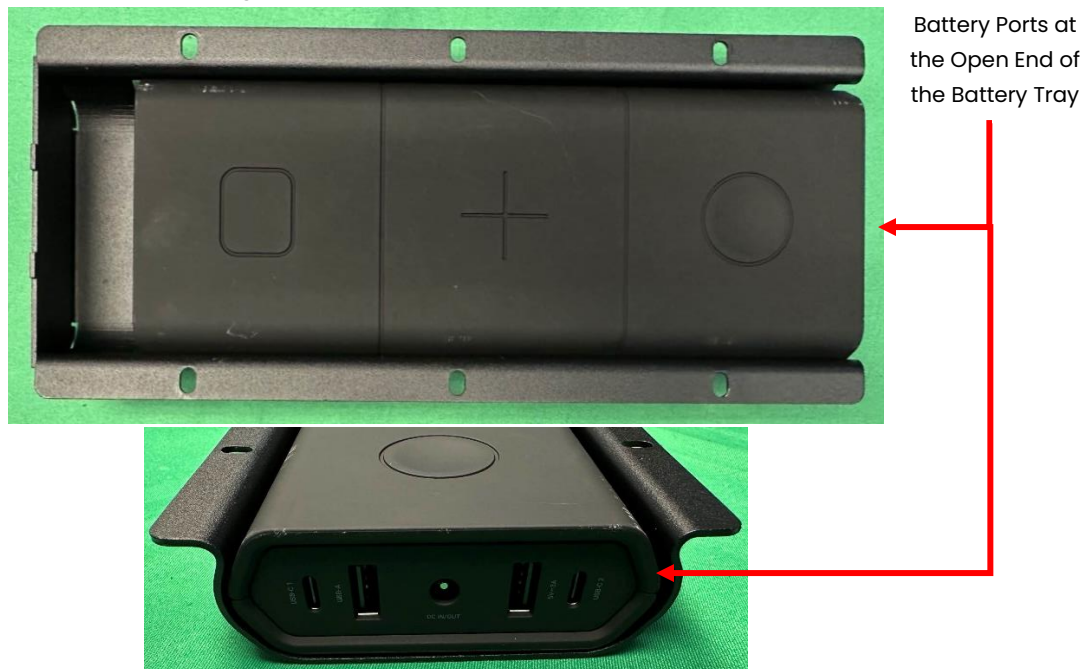
Figure 1: Place the Omnicharge 30C+ battery pack into the battery tray.
