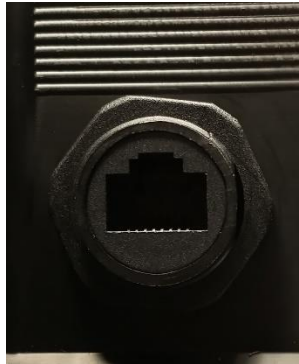
Figure 15: Connect the router to the RJ-45 ports on the case using ethernet cords.
