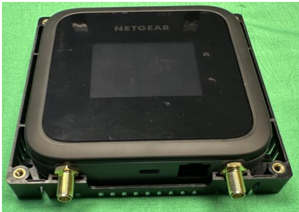
Figures 2-3: Installing the Router and Adapters to the M5-M6 Router Base and Cover
