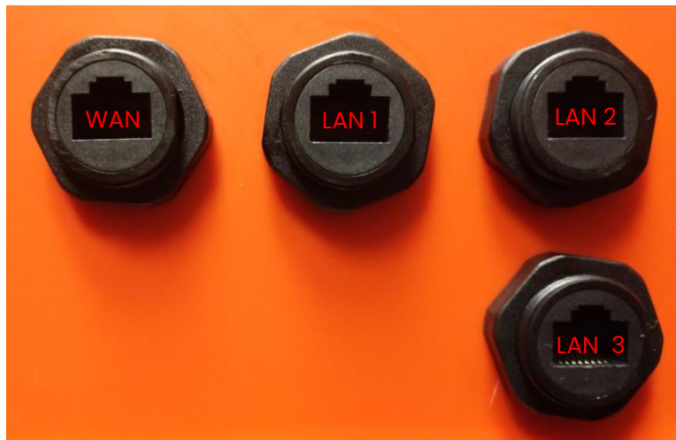
Figure 11: Connect the router to the RJ-45 ports on the case using ethernet cords.
