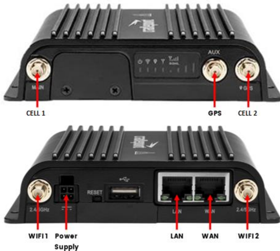
Figure 16: Cradlepoint IBR600 & IBR900 Connections
