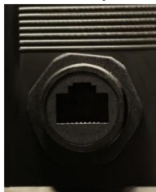
Figure 16: Connect the router to the RJ-45 ports on the case using ethernet cords.
