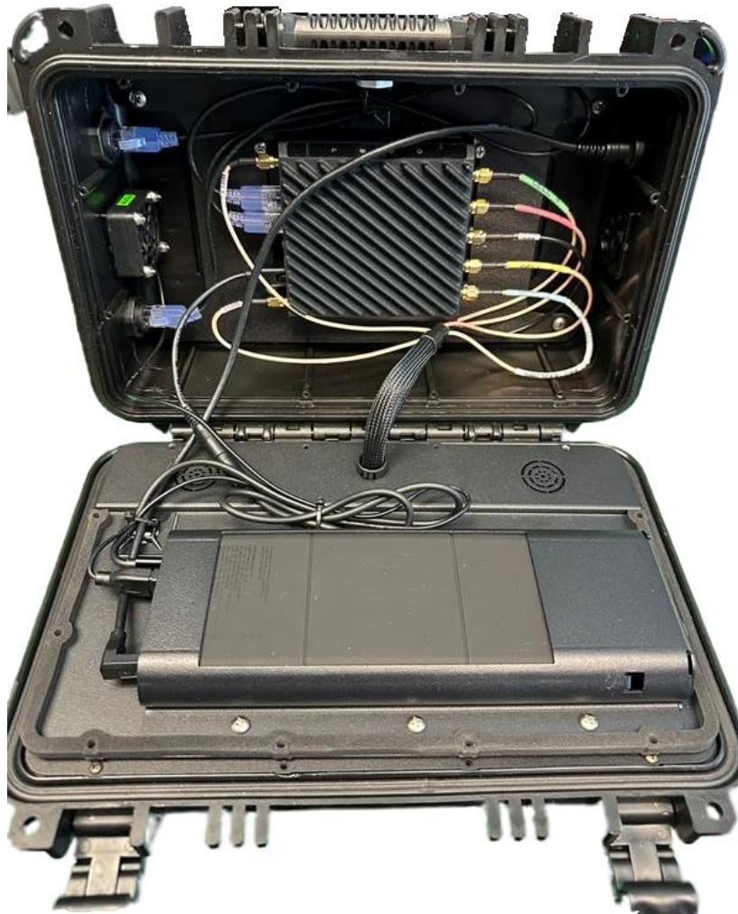
Figure 25: Fully Connected 7in1 Boxer R9 with Ericsson R9
