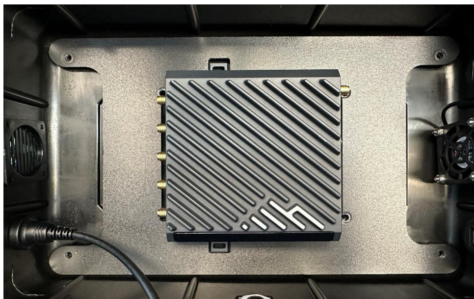
Figure 5: Place the PTA1111 Router Mount Plate with the foam on the underside
