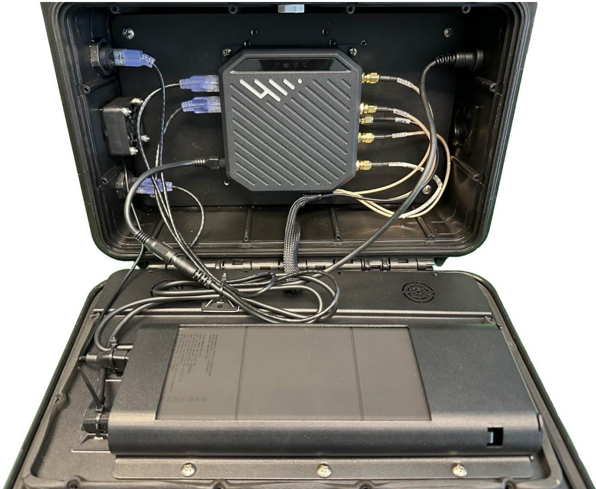
Figure 21: Fully Connected 5in1 Boxer G2 with Ericsson S700 Router
