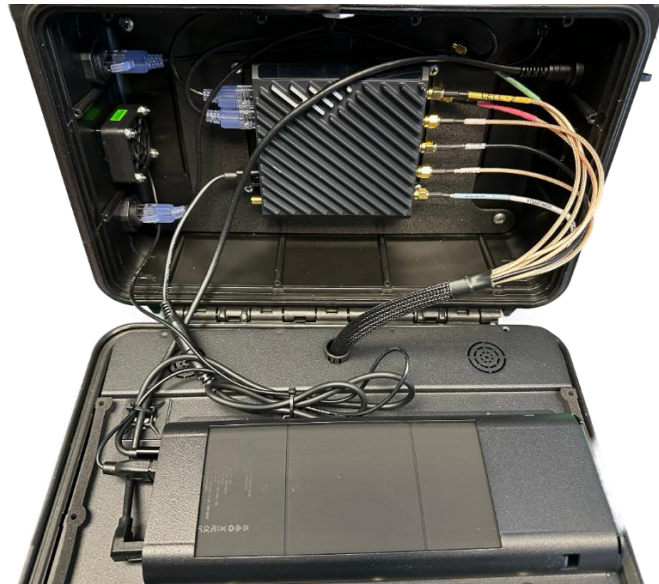
Figure 24: Fully Connected 5in1 Boxer R9 with Ericsson R920 Router
