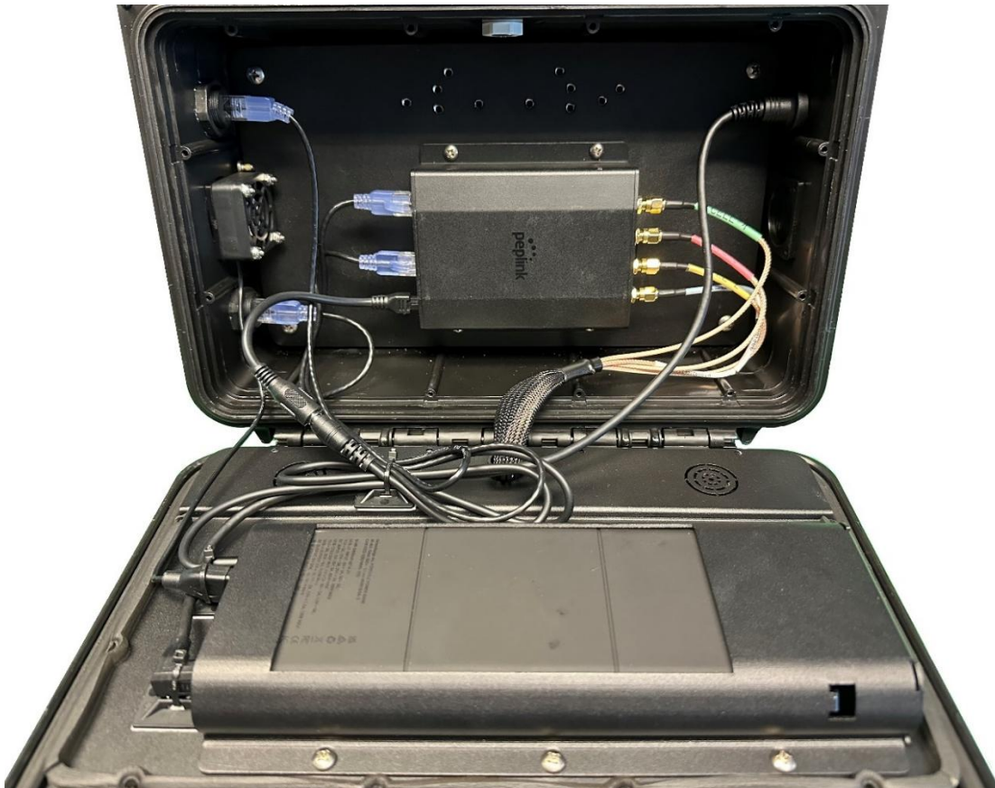
Figure 23: Fully Connected 4in1 Boxer G2 with Peplink MAX BR1 Mini Router
