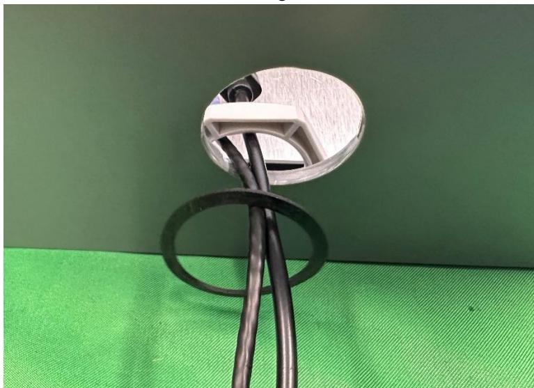
Figure 18: Feeding the gasket through the cable
