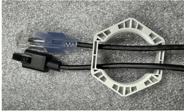
Figure 16: Feeding cables through cable gland nut
