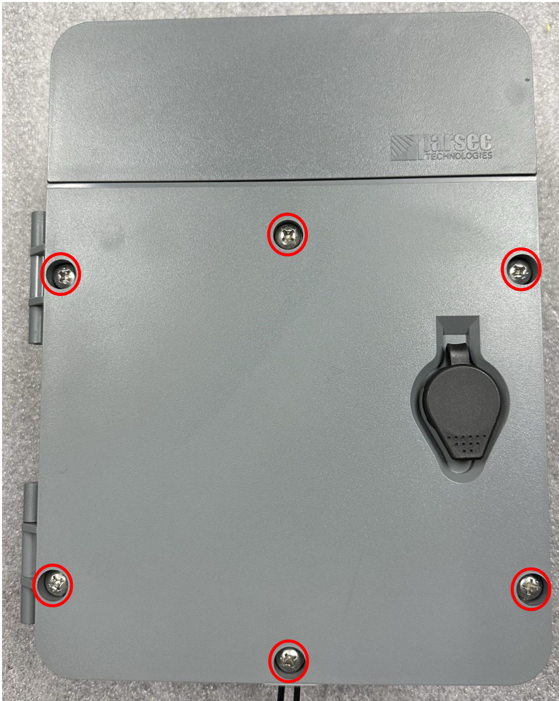
Figure 28: Fasten the lid to the enclosure
