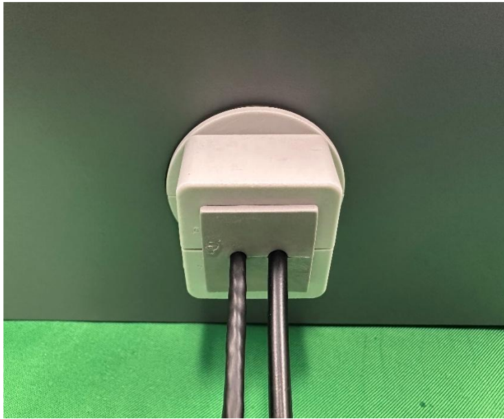
Figure 22: Installing the cable gland on the Mini-Dalmatian
